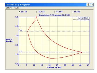
Pressure valve loss of ca. 31% in the 1st stage caused by too high gas pressure.
