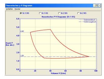
Suction and discharge valve losses of ca. 4% in the 1st and 2nd stage caused by too high gas velocity.
