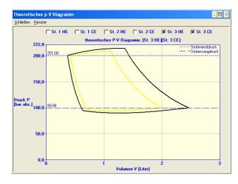
Valve problems in the 3<sup>rd</sup> stage caused by too high gas velocity.
