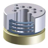
The PRValve differs from the poppet valve by using rings instead of poppets. This design improves the flow area by using two sealing faces per ring and the lift can be reduced which results in a lower impact.
